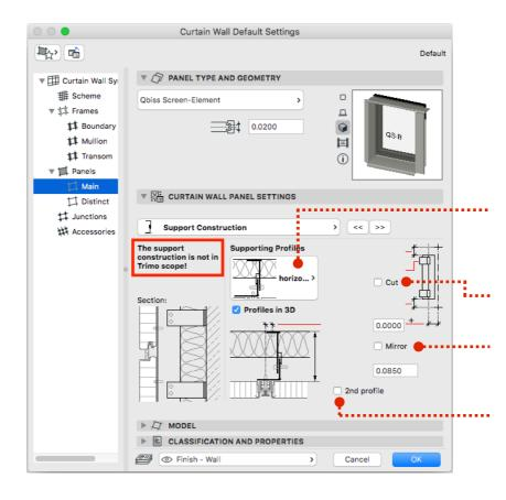
Depending on what system of elements you have choosen you get an option to select a horizontal or vertical support construction. You also have an option not having the support construction.
