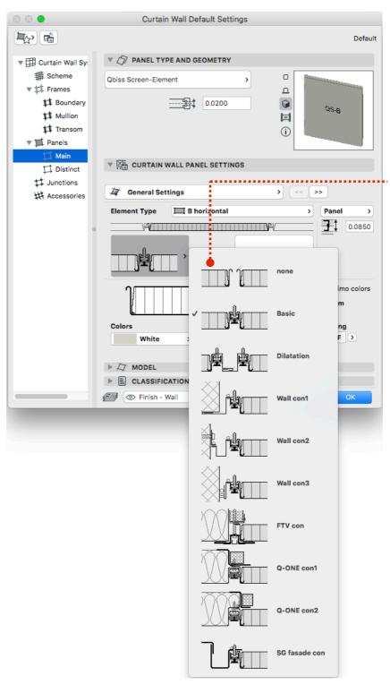
How the element connects to another element or wall.
